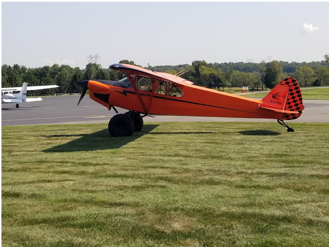
The large tires on the Piper Cub we saw at Sky Manor are Tundra Tires used for landing in rough areas (back country), allowing for more weight to be carried (including fuel) and better braking. Photos by Tony Marchand
