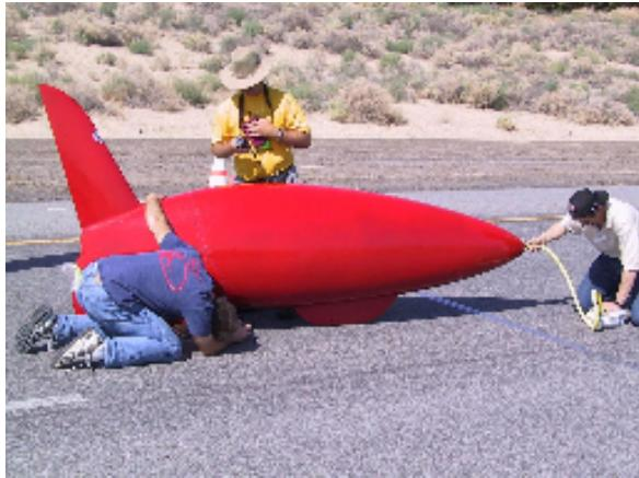
**All out performance is paramount.** The above vehicle is called a camera bike. A tiny camera mounted up on the tail fin gives the rider a view of the track on a small screen inside the shell. The reason is that windows trip the air flow from laminar to turbulent causing an increase in drag.
